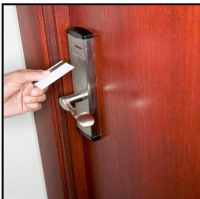
Many electronic access control locks use a Wiegand interface to connect the card swipe mechanism to the rest of the electronic entry system.
